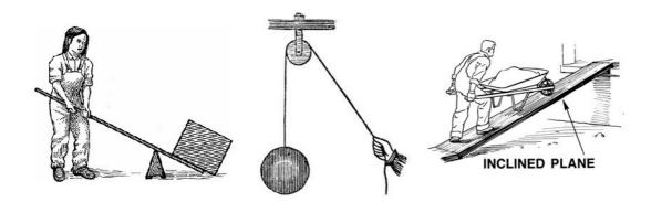
Some of the simplest machinesare the lever, the pulley and the inclined plane.
