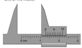
Look at the picture of the caliper. It marks 1,28 cm. To know it, you have to look at the 0 in the mobile scale (the superior one) which is between 1,2 and 1,3, but closer to 1,3. Now, look for the marks in both scales, superior and inferior, that are in the same position. In this case, is the eighth mark in the superior scale, so the value is 1,28 cm.
